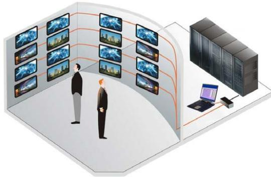
**Models** The UltraMatrix AV HD is available in a two models. The standard model has 16 HDMI inputs and 16 HDMI outputs. The second model adds a built-in LAN card to provide TCP/IP access to the unit.
