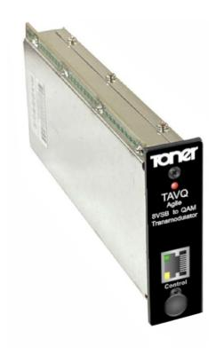
The TAVQ transcoder is a compact 8VSB to QAM transcoder that is packaged like any mini modulator and fits most standard mini mod chassis. The TAVQ features an 8VSB input frequency range of 54 to 806 MHz and QAM output frequency range of 54 to 1000 MHz. With the TAVQ you have the ability to edit PMT, Service / Network names as well as channel numbering in either virtual numbering or major / minor channel numbering. Setup is easily accomplished with an Ethernet connection and user friendly GUI.
